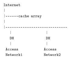
The DH scheduler can keep the two load balancer redirect requests destined for the same IP address to the same cache server. If the server is dead or overloaded, the load balancer can use cache\_bypass feature to send requests to the original server directly. (Make sure that the cache servers are added in the two load balancers in the same order)
