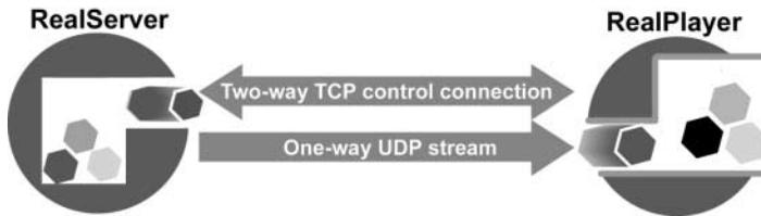
**How Clients Communicate with a RealServer from Behind a Firewall**
