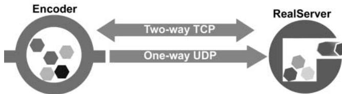
Some firewalls don't permit UDP packets, so RealProducer includes a setting that uses two-way TCP connections to send the same encoded content, as many firewalls do allow TCP traffic to pass through. This type of connection is illustrated in the following diagram.
