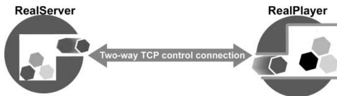
After the initial connection is established, RealServer then establishes a data channel back to the client. The actual media is sent along this channel, which uses UDP.
