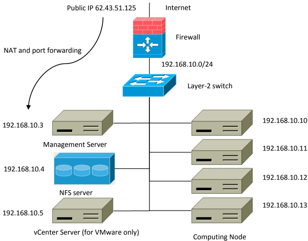
**Figure 1 Small-Scale Deployment**
