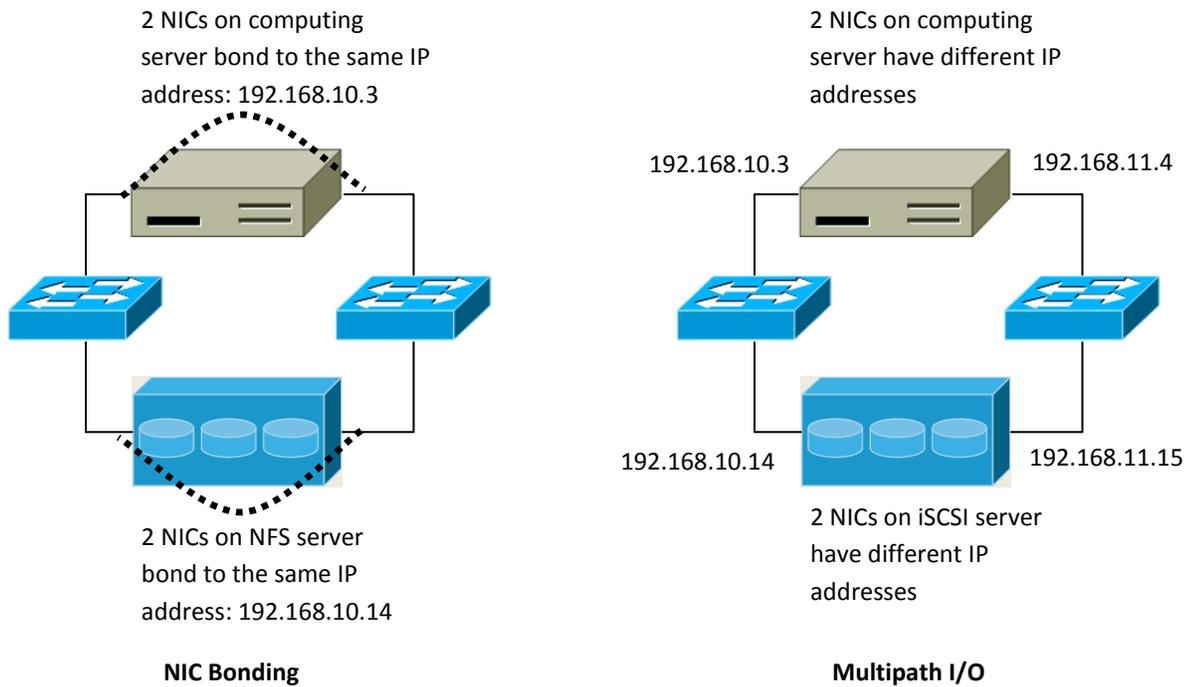
Figure 4 NIC Bonding and Multipath I/O
